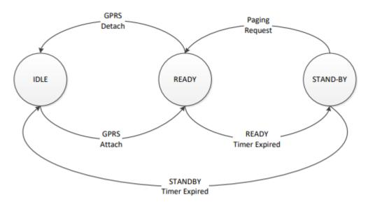
A test always starts and ends in the IDLE state, but reaching IDLE does not require compulsory stop (the test may continue). So, a test input consists of a sequence of events (E1, E2, ..., En), where E1="GPRS Attach" and En can be "GPRS Detach" or "STANDBY Timer Expired"."
